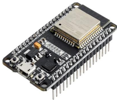
▼ 圖2-1 ESP32-WROOM DEVKIT V1
